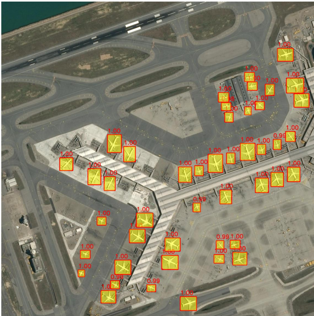
Fig. 2. Representative Output from Mask R-CNN Segmentation Results
