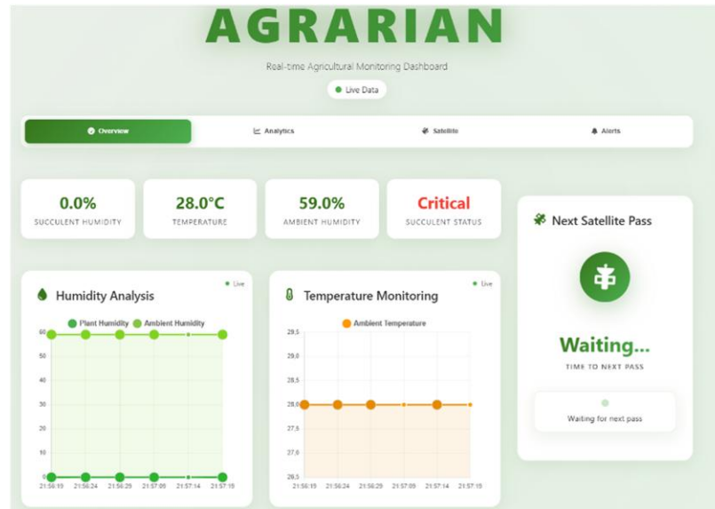
Fig. 7. Main dashboard interface with real-time crop monitoring.
