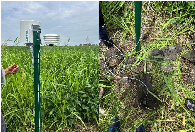
Figure 1. AGRARIAN in-field weather station installed in the Grivița pilot farm, used for real-time monitoring of climatic and soil parameters.
